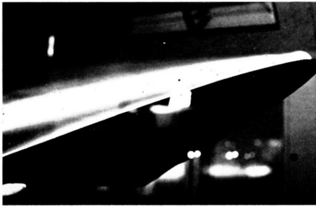
FIG. 6 — Visualisation of wing vortices by smoke flow
